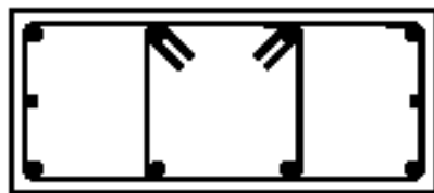
A1 30 \times 70 8\varnothing 20 + 2\varnothing 14
